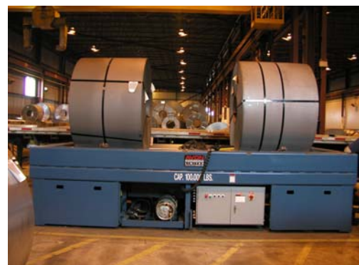
Propane powered master coil transfer car
