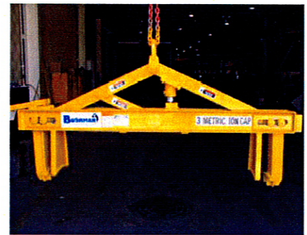
This three-ton supporting tong lifts rolls of steel belting.
