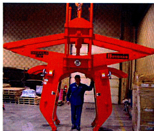
This 96,000 pound capacity tong lifts twin mill roll sets.
