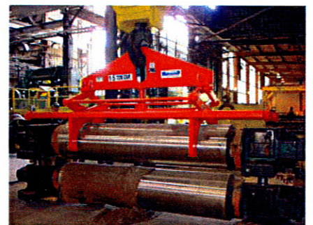
This roll tong lifts 22.5 to 25 inch diameter mill rolls. The legs have bronze wear pads to protect the roll surface.
